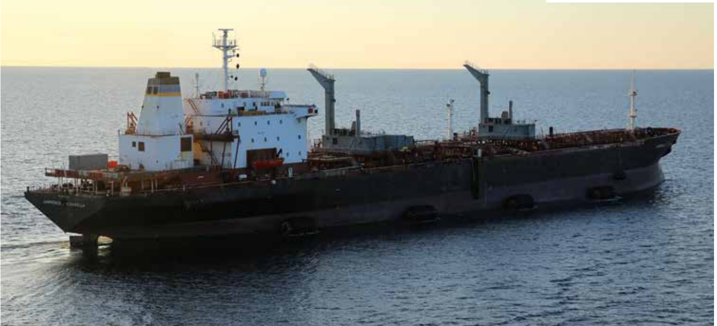
Military Sealift Command's petroleum tanker USNS Lawrence H. Gianella (T-AOT 112) pulls alongside the fleet replenishment oiler USNS Laramie (T-AO 203) while at sea. The ships came along-side each other to perform a skin-to-skin, fuel lightering operation. (U.S. Navy Photograph by Bill Mesta)
