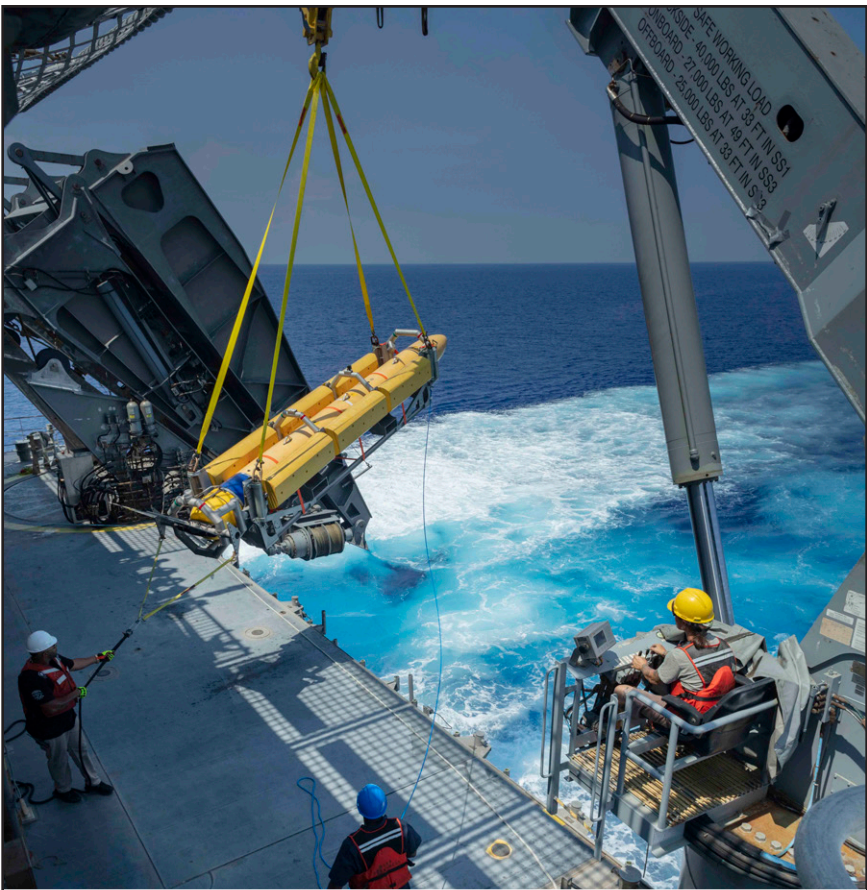
A Knifefish unmanned undersea vehicle (UUV) training model undergoes crane operations aboard the Military Sealift Command expeditionary fast transport vessel USNS Spearhead (T-EPF 1) as part of a training exercise enabling mine countermeasure missions (MCM) from an EPF as a vessel of opportunity. (U.S. Navy photo by Master-at-Arms 1st Class Alexander Knapp)
