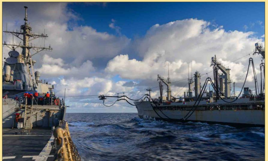
The Arleigh Burke-class guided-missile destroyer USS Fitzgerald (DDG 62) conducts an underway replenishment with the fleet replenishment oiler USNS Henry J. Kaiser (T-AO 187) in the Pacific Ocean, Jan. 27, 2025. Fitzgerald is underway in the U.S. 3rd Fleet conducting routine operations. (U.S. Navy photo by Mass Communication Specialist 1st Class Jesse Monford)
